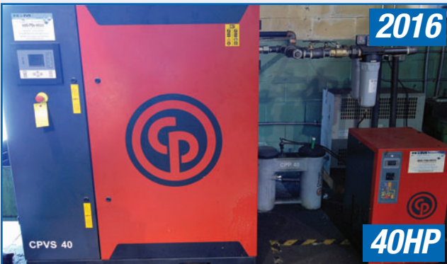
CHICAGO PNEUMATIC CPVS40 COMPRESSOR W/ DRYER
